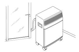
b) through a small hole 2.16" x 0.98" (2.5 cm x 5.5 cm) drilled in the lower part of a door or in a window frame by using the frame provided.
